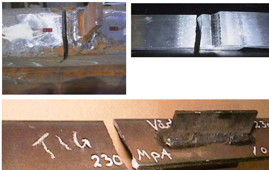
Figure 133 - Examples of laboratory fatigue tests in which weld improvement has led to eventual failure away from the weld detail [64] [67].
