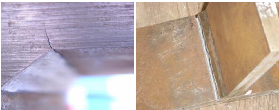
Figure 41 – Typical failed specimens - Crack initiating at the weld toe
