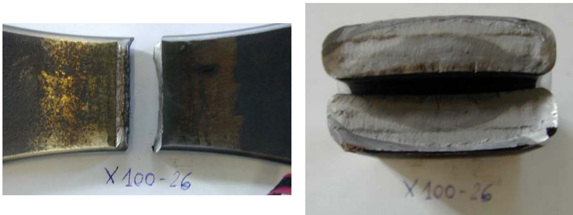
Figure 45 – Typical failed specimen and fracture surface appearance
