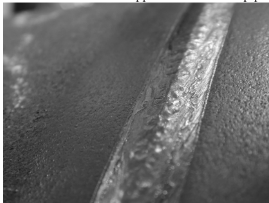
Figure 191 –Weld cap appearance on X100 pipes 16.4 mm thick.
