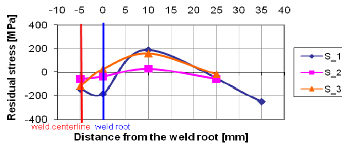
Figure 32 – X100 FCAW - Residual stresses on internal surface in longitudinal direction measured on two samples S_1, S_2.
